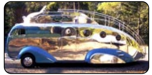
Randy Grubb's Decoliner Flash Gordon's Motorhome. This 26-foot polished aluminum beauty features a flying bridge, complete with driving station and room for 5 passengers on the roof. It uses the chassis from a 1973 GMC Motorhome and a 1955 White cab-over engine.
