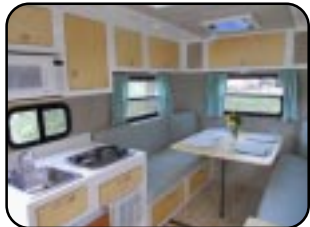
The ParkLiner interior showing the sink, stove and dinette area with the "Magic" table set up full size.
