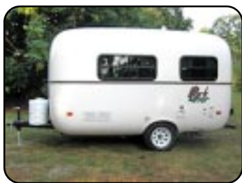
The ParkLiner features a two part fiberglass shell a frame supported by a 3,500 lb axle and 14-inch wheels.
